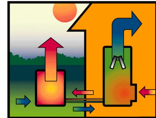
During the summer, heat is extracted from the home by passing indoor air across a refrigerant coil in the inside unit. The heat is then carried by lines to the outside unit, where it is released to the outside air which cools your home.
