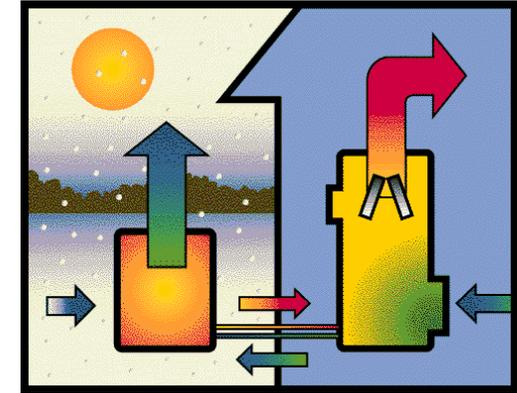
During the winter, the outside coil absorbs heat from the outside air and transfers it via refrigerant lines to the inside coil, where it is released to warm your home. An auxiliary (back-up) electric resistance heater works with the heat pump when the outdoor temperature goes below the balance point.
